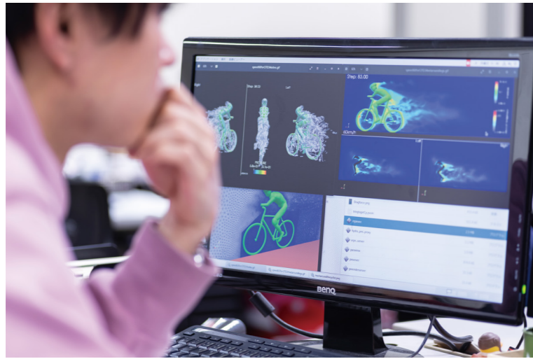
Simulating the flow field around a bicycle and predicting optimal pedaling motion
