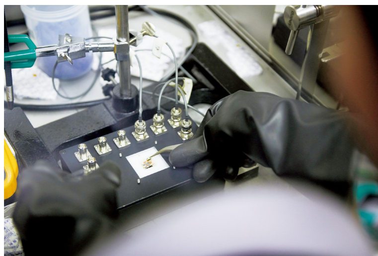
Preparing for the measurement of organic semiconductor devices in a nitrogen glove box
