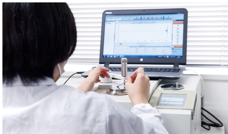
Analysis via Fourier Transform Infrared Spectroscopy (FTIR) with an attenuated total reflectance (ATR) attachment
